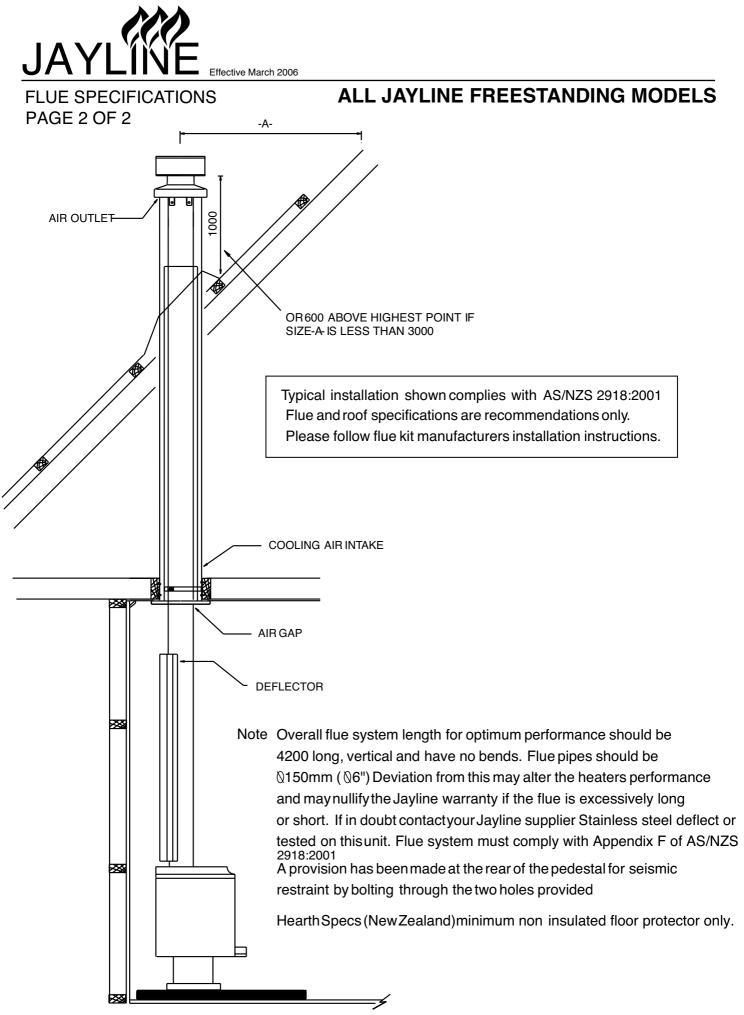
IF INSTALLED IN ACCORDANCE WITH THESE SPECIFICATIONS THE HEATER COMPLIES WITH AS/NZS 2918:2001 including appendix F
