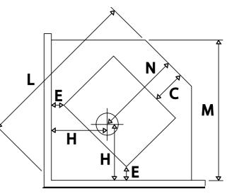
Dimension 'C' is taken from door seal lip (fire box) to the front of the floor protector. All dimensions are in millimetres. All dimensions are set as a minimum guide only.
